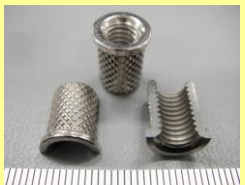
Cold Heading + Rolling + Tapping Combination
